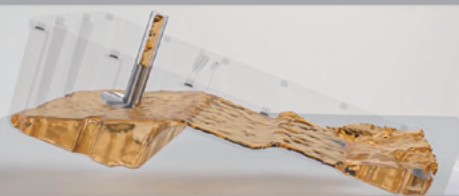
Oil pan sloshing simulation
